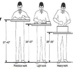
The diagram illustrates three standing workstations. The first is for 'Precision work' with a height range of 37-43 inches. The second is for 'Light work' with a height range of 34-37 inches. The third is for 'Heavy work' with a height range of 28-35 inches. Each workstation shows a person with their arms resting on the work surface.
