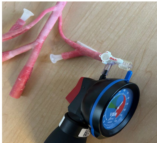
Alternate option for direct stopcock insertion for balloon inflation and pressure monitoring.
